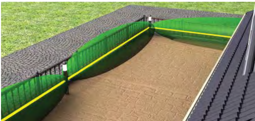
Protection of the perimeter using Dual Technology Bistatic sensor FORTEZA-FONAR-COMBI
