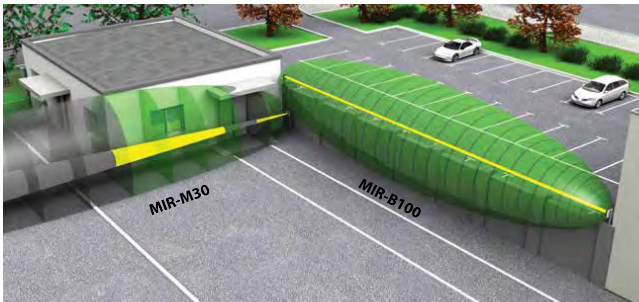
Protection of the perimeter using the Dual Technology Bistatic sensor MIR-B100 and Dual Technology Monostatic sensor MIR-M30
